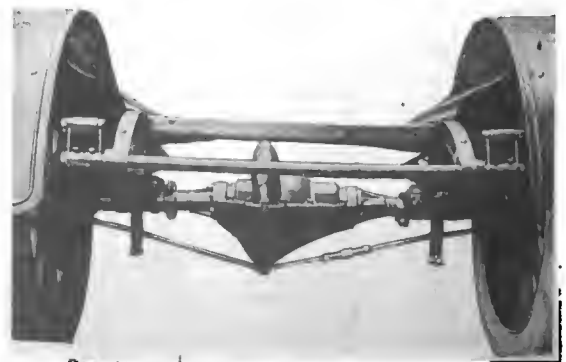
Rear View, Showing Ball Bearing Floating Axle.
